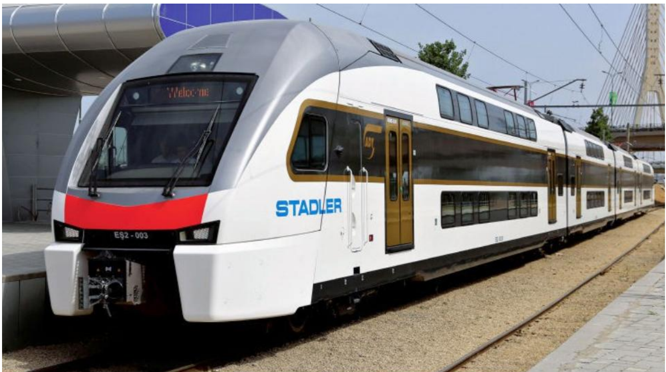
Figure 4-1: Regional rapid transit utilises short double decker trains to not interfere too much with freight services in the same corridor
